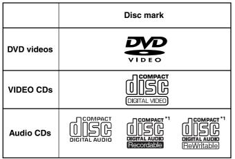
\*1 This unit can play CD-R and CD-RW discs recorded in CD Audio or Video CD format, or with MP3 audio files.
