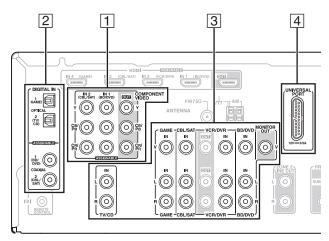
Connect your components to the appropriate jacks. The default input assignments are shown below.
