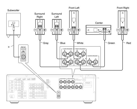
\* Using the supplied RCA cable, connect the subwoofer's LINE INPUT to your AV receiver's SUBWOOFER PRE OUT.
