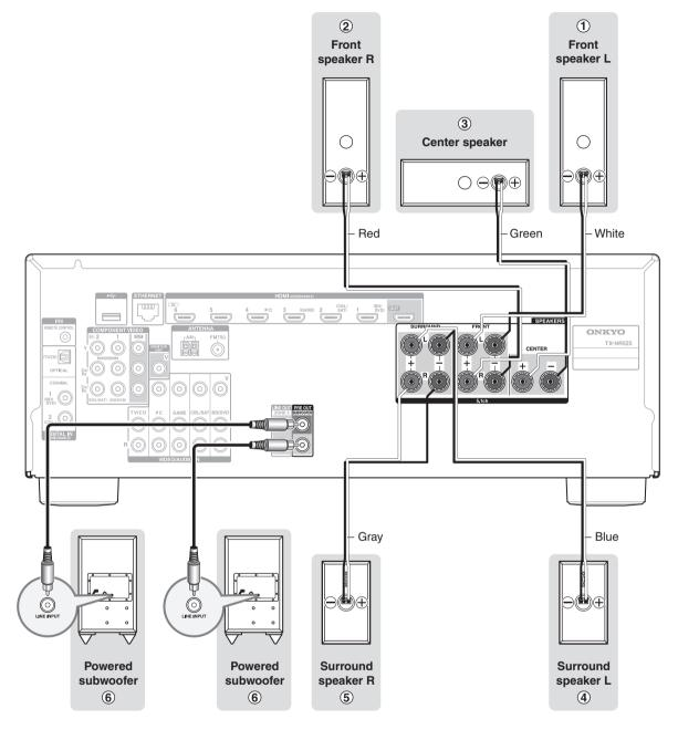
You can connect the powered subwoofer with two **SUBWOOFER PRE OUT** jacks respectively. The same signal is output from each jack.
