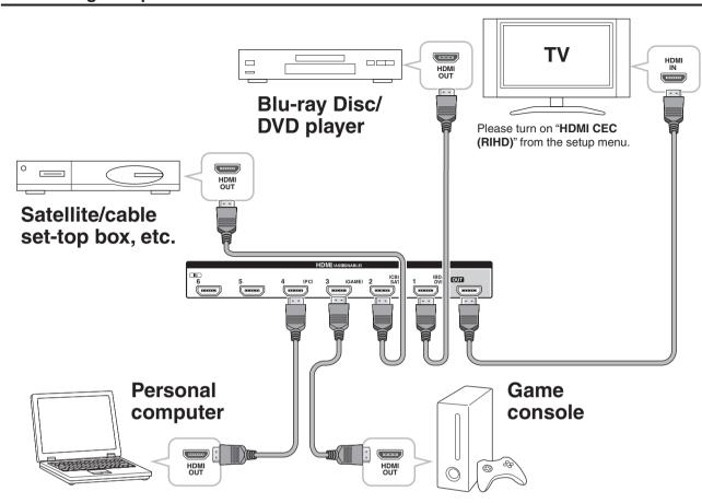
The components connected to each terminal (BD/DVD, GAME, etc.) can be selected with the input selector buttons of the same name on the front panel. Note that these default assignments can be changed. For details, please refer to the instruction manual.
