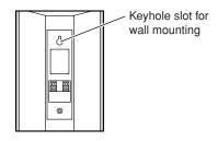
To mount the center speaker horizontally, use the two keyhole slots shown to hang each speaker on two screws that are securely screwed into the wall.
