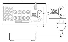
Make sure that the maximum power requirement of the component connected to the AC OUTLET does not exceed the capacity printed on the A-933's rear panel (100W).
