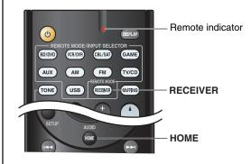
To reset the remote controller to its factory defaults, while holding down **RECEIVER**, press and hold down **HOME** until the remote indicator lights (about 3 seconds). Within 30 seconds, press **RECEIVER** again.
