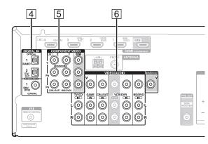
Connect your components to the appropriate jacks. The default input assignments are shown below. See "Connection Tips and Video Signal Path" for more information (→ page 57). The on-screen menus appear only on a TV that is connected to the HDMI OUT. If your TV is connected to other video outputs, use the AV receiver's display when changing settings.
