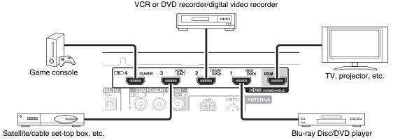
\* If your TV doesn't support Audio Return Channel (ARC), you need to connect an optical digital cable together with the HDMI cable to the AV receiver.
