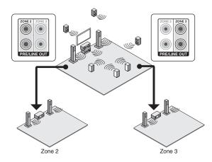
Volume can be adjusted with both the unit and the premain amplifier used in a separate room. To adjust it with the unit, press RECEIVER and then HOME on the remote controller, select "Setup" - "7. Hardware Setup" - "Multi Zone" - "Zone 2 Out" or "Zone 3 Out" and set the setting to "Variable". If you connect a power amplifier, be sure to make the setting and adjust the volume in the main room.
