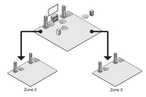
Required setting: Press RECEIVER and then HOME on the remote controller. Select "Setup" - "2. Speaker Setup" - "Speaker Settings" and set "Powered Zone 2" or "Powered Zone 3" to "Yes".
