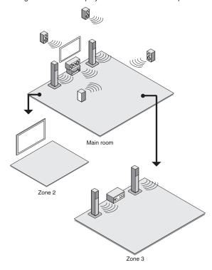
● The sources from which you can enjoy the sound in a separate room: For Zone 2, any can be selected from among an external device connected to the HDMI input jack or the analog audio input jacks (\*) of the unit, the "NET", "USB" or "BLUETOOTH" source, and the AM/FM
