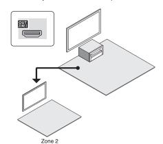
Change the setting: Press RECEIVER and then HOME on the remote controller, select "Setup" - "1.Input/Output Assign" - "Monitor Out" - "Zone 2 Monitor Out" and set the setting to "Use".
