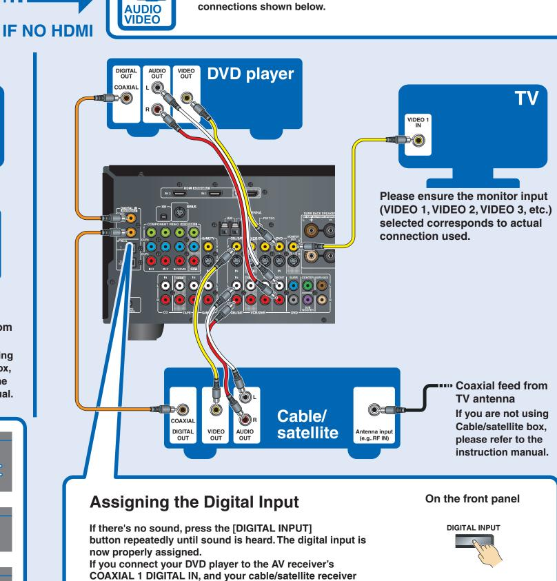
to the COAXIAL 2 DIGITAL IN, as shown, it's not necessary to assign the digital input.
