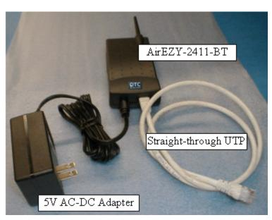
*properly when connected to a hub plugged in with multiple computers/network-devices.* So as a rule, straight-through cable is always used to connect an AirEZY-2411-BT Station to a computer or a network device.
