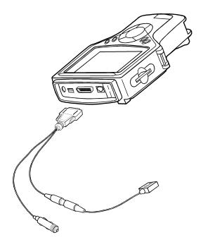
Figure 2.11: DB25 Power Cable Connection to NGIS Tool
