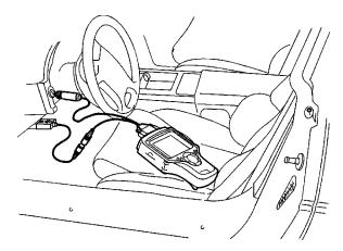
Figure 2.13: DB25 Power Cable Connection to Vehicle's DLC
