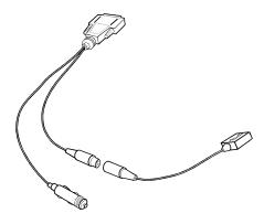
Figure 2.10: Adapter Connection to DB25 Power Cable
