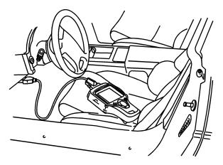
Figure 1.1: NGIS Tool Connected to Vehicle DLC
