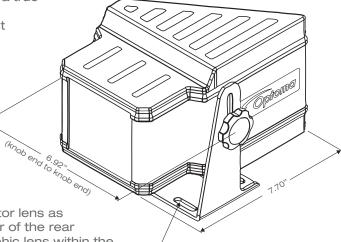
Four bracket mounting slots accept 1/4" screws
