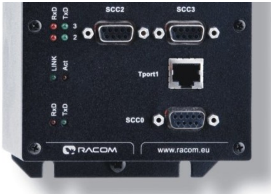
Fig. 3.10: T-port module on the 2nd slot of the modem
