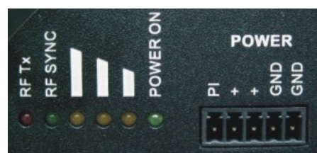
Fig. 3.12: Power connector & information LED
