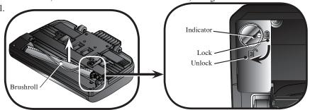
**IMPORTANT:** Rotate screw 1/4 turn until the indicator is aligned with the "unlock" symbol.
