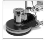
Lean handle back. While handle is released and with both hands on handle grips, squeeze the ON/OFF lever located on the right grip to turn on
