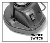
the outlet. Before turning machine on, be sure there is a pad or brush in place on the machine. Note - do not kick switch. Gently activate the switch with your toe. No force is necessary.
