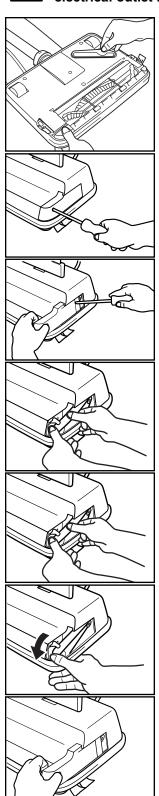
Remove the replacement belt from the storage channel.
