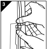
Before assembling appliance, remove two screws from connector assembly. Remove cardboard insert by pulling upward (fig 1).
