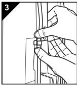
Attach cord to cord clip by pressing cord above and below clip ensuring the cord is fully rested in clip.
