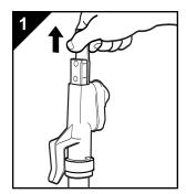
Before assembling appliance, remove two screws from connector assembly. Remove cardboard insert by pulling upward.
