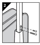
With ON/OFF switch facing the front of the unit, slide upper handle section over matching section of the connector assembly. Insert short screw into top hole and long screw into bottom hole then tighten firmly until handle is no longer loose.
