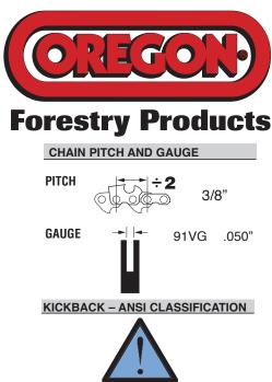
91VG saw chain is a low kickback saw chain. It met the kickback performance requirements of ANSI B175.1 (USA), and CSA Z62.3 (Canada) when tested on a representative sample of chainsaws. Its safety features significantly reduce the hazard of kickback while maintaining high cutting performance. ALL CUTTING SAW CHAINS CAN KICKBACK, which may result in severe personal injury to the saw operator or bystanders. Operate your saw safely. Read all warnings in your chainsaw operator's manual.
