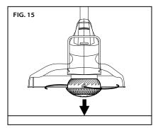
If the trimmer line does not come out, the spool may be empty. Turn off the trimmer/edger and replace trimmer line as described in "Replacing trimmer line".
