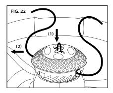
• Hold the trimmer head with one hand and turn the knob counter-clockwise to wind the line until about 13–15 cm (5–6 in) of line protrudes from each eyelet (Fig. 23).
