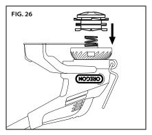
• Line up the tabs on the cover (1) with the slots in the trimmer head (2), and press the cover onto the trimmer head until both tabs click into place. (Fig. 27).
