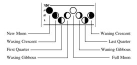
To check the moon phase for a particular day, press the UP or DOWN button once. The clock will enter moon phase scanning mode.
