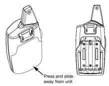
Insert the batteries observing the correct polarity as marked inside the battery compartment.
