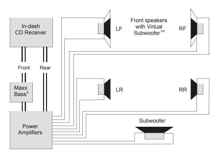
**WARNING:** If you are using a source unit with bridged high powered (or "floating ground") speaker outputs, a suitable high to low level adapter must be used. If you are unsure about your head unit see your local **Orion** dealer.
