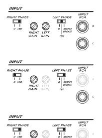
BRIDGE 180 Setting 4 inverts the output of both the left and right channels. Both left and right gain controls are active. This configuration is useful for inverting one set of speakers like rear speakers in front/rear system to improve staging in a vehicle.
