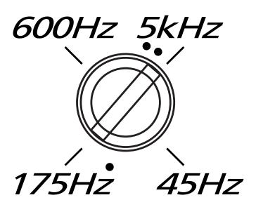
The crossover section is marked at four frequency points for ease of system adjustment. These points are 45 Hz, 175 Hz, 600 Hz and 5,000 Hz. Specific crossover points can be to be chosen based on the recommended operational bandwidth of your speakers.
