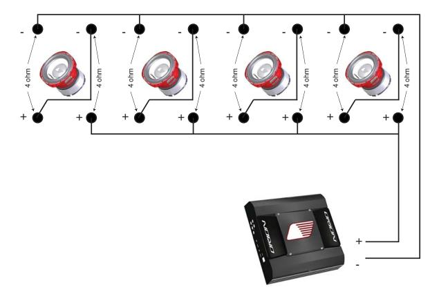
1. Connect each woofer in series by connecting the negative (-) of the first coil to the positive (+) terminal of the second coil.
