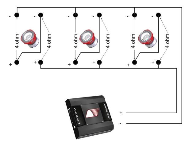
1. Connect each woofer in series by connecting the negative (-) of the first coil to the positive (+) terminal of the second coil.
