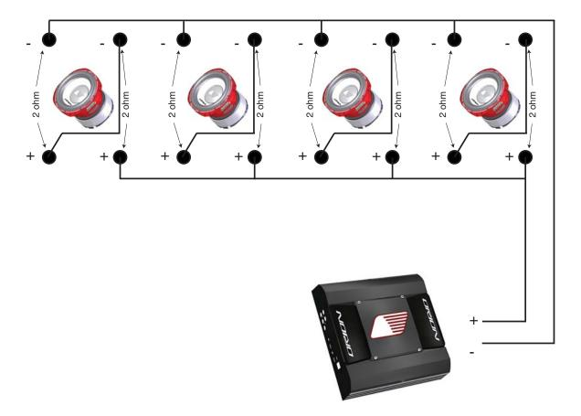
1. Connect each woofer in series by connecting the negative (-) of the first coil to the positive (+) terminal of the second coil.
