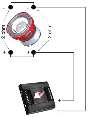
1. Connect the speaker in parallel by connecting the two positive (+) terminals together and the two negative (-) terminals together.
