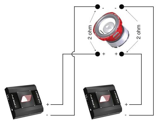
1. Connect one of the speaker's voice coils to the first amplifier by connecting the positive (+) terminal and the negative (-) terminal from the speaker to the respective positive (+) terminal and the negative (-) terminal from the first amplifier.
