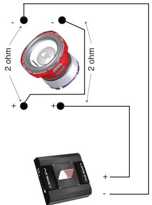
1. Connect the woofer in series by connecting the negative (-) of one terminal to the positive (+) terminal of the other coil.
