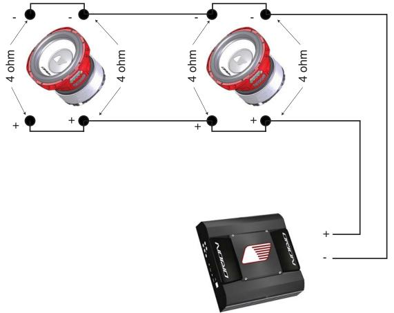
1. Connect the speaker in parallel by connecting the four positive (+) terminals together and the four negative (-) terminals together.
