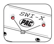
Once programming is completed, wait 7 seconds. Both LEDs will flash three times indicating end of programming. The Interface will then flash the version number it was programmed for.
