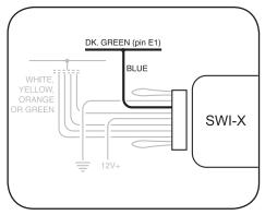
Note: **Step 4a** is for vehicles made by General Motors that are programmed for version #4 only. If no connections is necessary, proceed to Step 4b.
