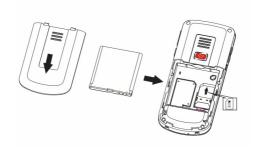
Observe the battery contacts (the gold coloured contacts must face towards the bottom right).and insert the battery.
