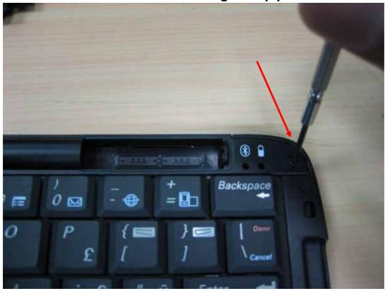
Remove the strip panel by releasing the snap hook
