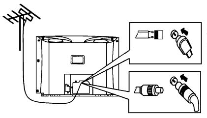
Note: In case of using the Twin-lead aerial feeder (300 $\Omega$ ) for UHF/VHF aerial, use a 300-75 ohm adaptor (not supplied)
