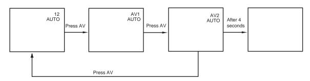
Note: S-VHS IN and AV2 use the same interface. If you want to receive signals input through S-VHS terminal, switch the set to AV2, the S-VHS (S-VIDEO) input terminal has priority over the AV2 VIDEO terminal; To use equipment connected to the AV2 VIDEO IN terminal, disconnect any plug from the S-VHS terminal. S-VHS and AV2 use the same group of AUDIO IN terminals.
