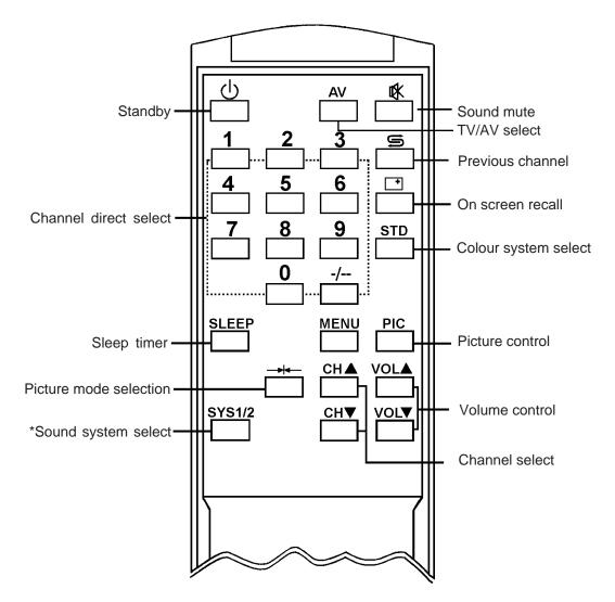
\* NOTE: this TV model's RF sound system is BG only. Therefore the **SYS1**/2 button on the remote controller is ineffective in sound system selection. Similarly in the **Preset** and **Function** menus the **SYS** item (sound system selection item) is ineffective.
