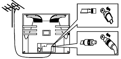
Note: In case of using the Twin-lead aerial feeder  $(300\Omega)$  for UHF/VHF aerial, use a 300-75 ohm adaptor (not supplied)
