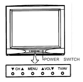
Note: Functions of  $\blacktriangle$  CH  $\checkmark$ , MENU,  $\bigstar$  VOL  $\checkmark$ , TV/AV are also provided to the remote controller.
