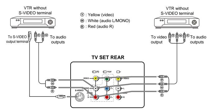
To access the unit connected to these jacks, press TV/AV button until AV1 or SVHS appears on the screen.
