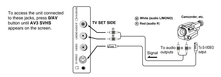
Note: The S-VIDEO input terminal has priority over AV3 VIDEO terminal. To use equipment connected to AV3 VIDEO terminal, disconnect any plug from the S-VIDEO terminal.
