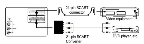
**Note:** If the equipment you want to connect is not equipped with 21-pin Scart, you can connect it by using the **21-pin Scart Convertor** (supplied) as illustrated above.
