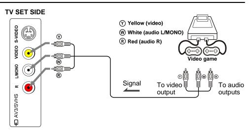
The figure below shows how to connect the SVHS input to video equipment.
