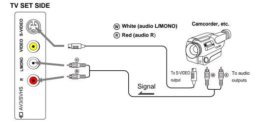
Note: The S-VIDEO input terminal has priority over AV3 VIDEO terminal. To use equipment connected to AV3 VIDEO terminal, disconnect any plug from the S-VIDEO terminal.
