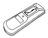
Insert two size AAA batteries according to the polarity indication inside the remote controller.
