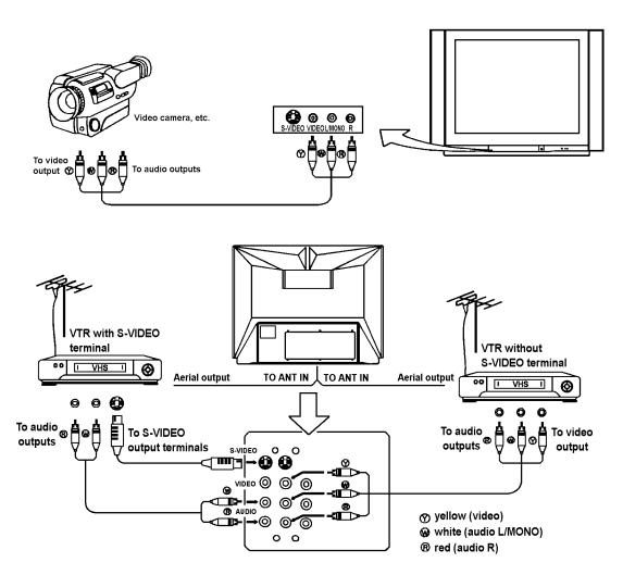
To select the input press the AV button on the remote controller repeatedly until you see the corresponding input indication on the screen. To return to aerial input, press the AV button until it displays programme number, or press direct channel select button or the CH ▲/▼ button.
