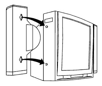
Loosen the screws to remove the speaker from the TV
