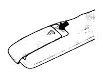
1 Remove the cover of the remote controller by pressing the symbol and pulling the cover space in the direction of the arrow.
