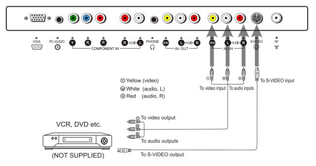
Note: Composite video is the most common used signal, but the picture quality is not as high as S-video.
