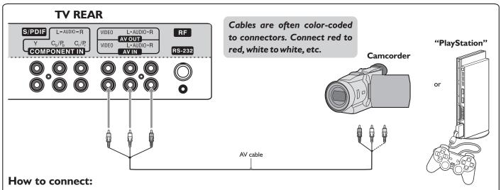
Connect the Audio/Video cables between the Audio (L/R)/Video jacks on the unit and camcorder.
