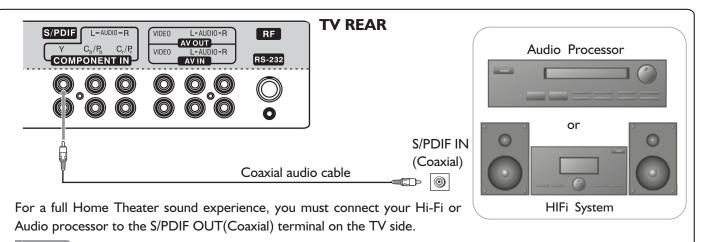
Note The S/PDIF OUT jack is available only when a digital TV channel is received.
