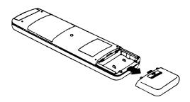
2) Insert two size AAA batteries according to the polarity indication inside the remote controller.
