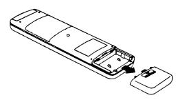
Insert two size AAA batteries according to the polarity indication inside the remote controller.
