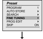
In **FINE TUNING** sub-menu, press **P-** or **P+** to select **TUNING**, then press and hold **V+** or **V-** to fine tune to obtain best possible picture and sound.
