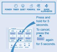
To switch the temperature setting to °C or °F, press and hold for approximately 10 seconds.
