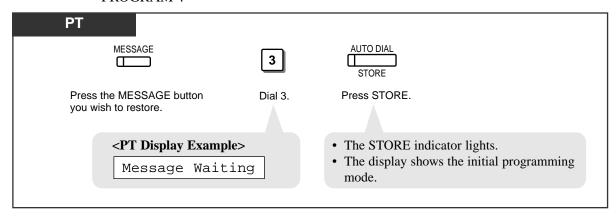
— To exit the Station Programming mode, set the MEMORY switch to "SET".
