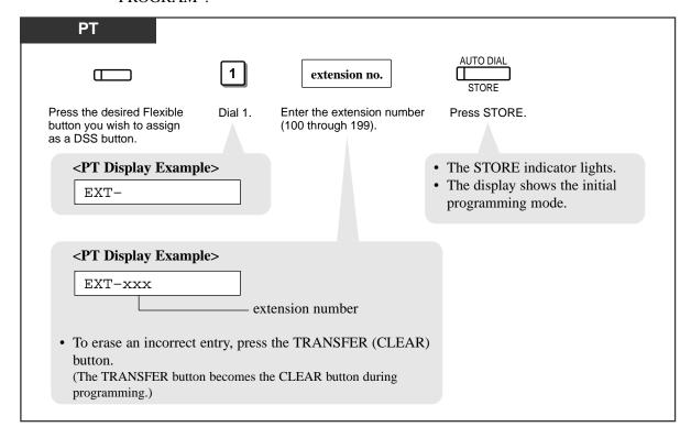
— To exit the Station Programming mode, set the MEMORY switch to "SET".
