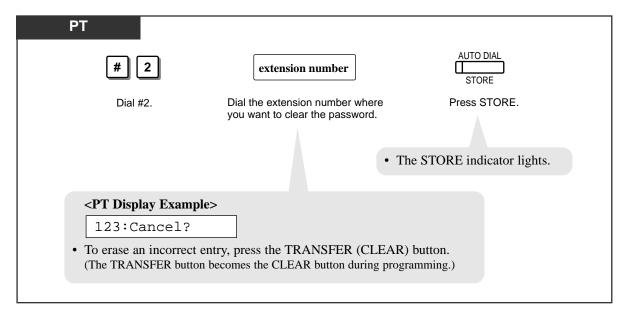
— To exit the Station Programming mode, set the MEMORY switch to "SET".
