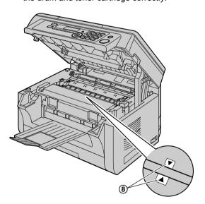
6 Close the top cover by holding the indentations on both sides of the unit, until locked.
