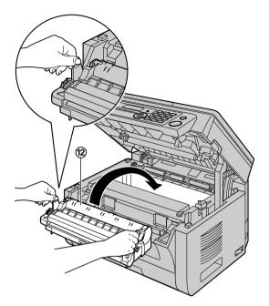
Make sure that the arrows (③) match, to install the drum and toner cartridge correctly.
