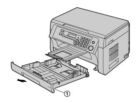
2 Before loading a stack of paper, fan the paper to prevent paper jams.
