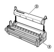
4 Press down the toner cartridge firmly (⑤). Keep pressing while turning the green lever on each side of the toner cartridge towards you (⑥).
