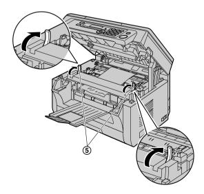
Remove the jammed paper (6) carefully by pulling it upwards.
