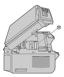
7 Install the drum and toner cartridge (②) by holding the tabs.
