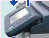
2nd Position (Ex: Use the 2nd or 3rd position when the reflection from the overhead light interferes viewing the panel.)
