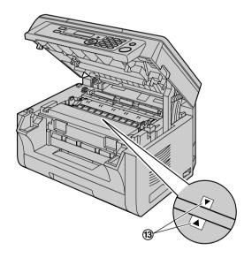
8 Close the top cover by holding the indentations on both sides of the unit, until locked.
