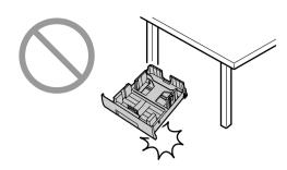
Hold the paper input tray with both hands when removing or installing. The paper input tray weighs approximately 2 kg when fully loaded with recording paper.
