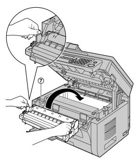
Make sure that the arrows (®) match, to install the drum and toner cartridge correctly.
