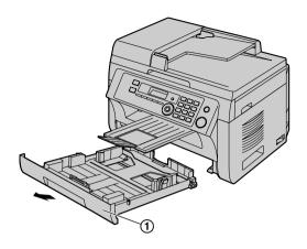
2 Before loading a stack of paper, fan the paper to prevent paper jams.
