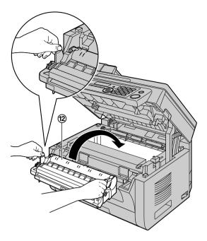
Make sure that the arrows (<sup>(3)</sup>) match, to install the drum and toner cartridge correctly.
