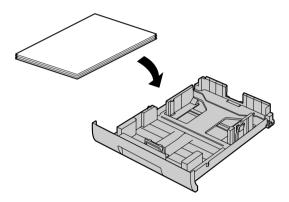
3 Insert the paper input tray into the unit, lifting the front part of the tray. Then push it completely into the unit.
