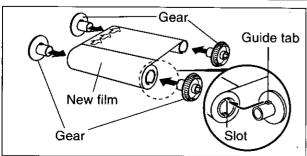
Insert the four gears into the new film cores so that the guide tab of each gear fits into the slot of the film core.
