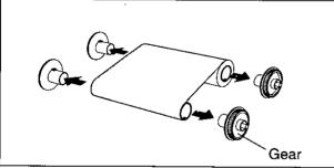
6 Pull out the four gears from the used film cores.
