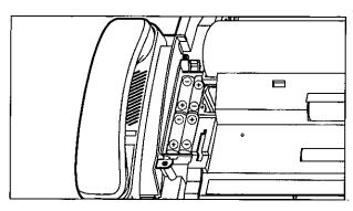
Install four batteries into the compartment using correct polarity (+, -).
