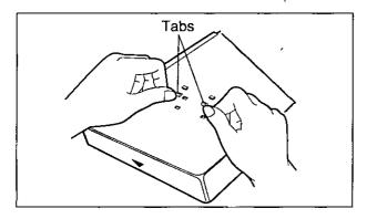
Turn over the cassette and remove the partition by pushing the lower two tabs of the partition.
