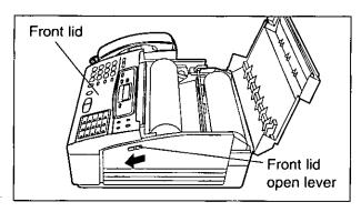
Open the top cover, then open the front lid by sliding the lever towards you.
