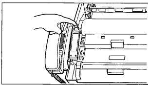
2 Remove the battery compartment cover by pulling the hook towards you and lifting it up.
