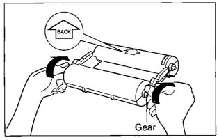
Place the cartridge with the "BACK" indicator facing up and tighten the film by winding the gears if there is slack.
