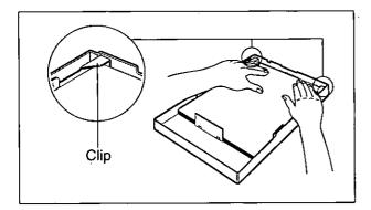
Push down the opposite edges so they are secured under the clips.
