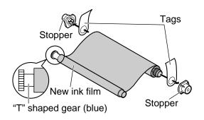
Insert the blue core of the front ink film roll into the right slot of the unit (1). Insert the "T" shaped gear (blue) into the left slot of the unit (2).
