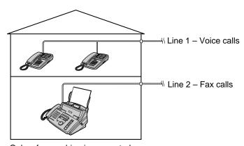
Only a fax machine is connected.
